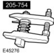
Ball joint separator 205-754 (LRT-54-027)
